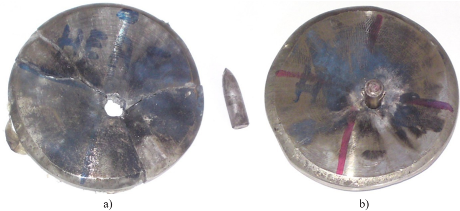
Fig. 5. The impact behaviour of HEA plates before and after heat treatment
