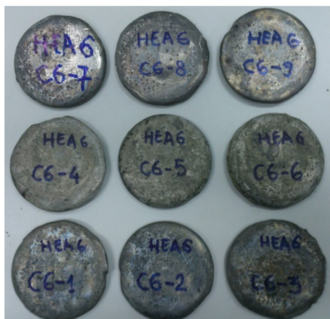
Fig. 1. As-cast HEA samples from AlCoCrFeNi alloying system
