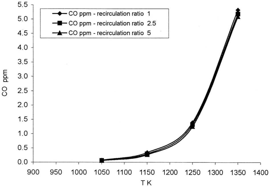
Fig. 9. Final CO concentration as a function of air temperature
