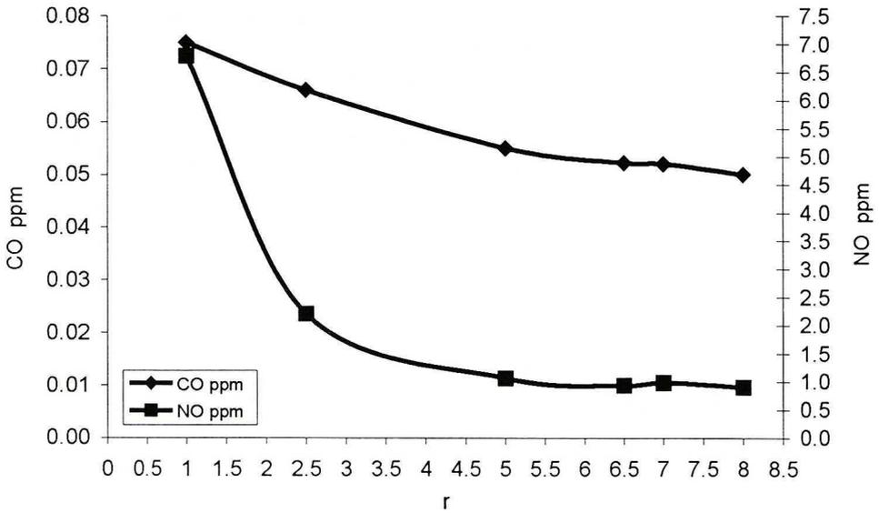
Fig. 5. Calculated final CO and NO concentrations as functions of recirculation rate  $r$  for air temperature 1050K
