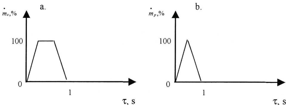
Fig. 4. Assumed, relative mass fluxes of recirculation gases (Fig. a) and fuel (Fig. b) as functions of time
