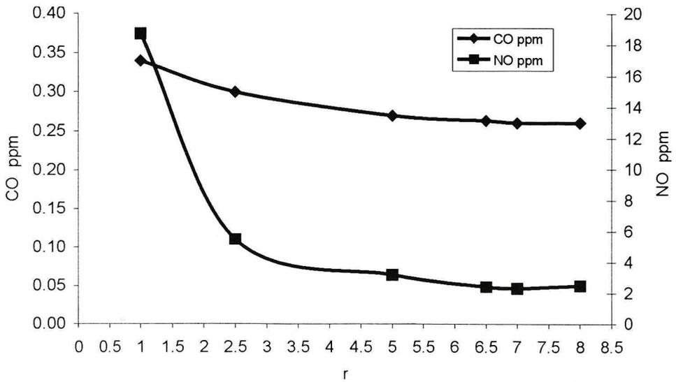
Fig. 6. Calculated final CO and NO concentrations as functions of recirculation rate  $r$  for air temperature 1150K
