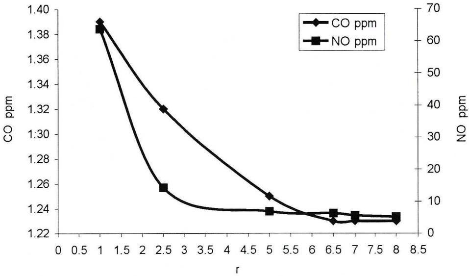
Fig. 7. Calculated final CO and NO concentrations as functions of recirculation rate  $r$  for air temperature 1250K
