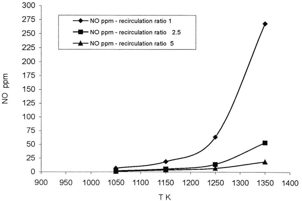
Fig. 10. Final NO concentration as a function of air temperature
