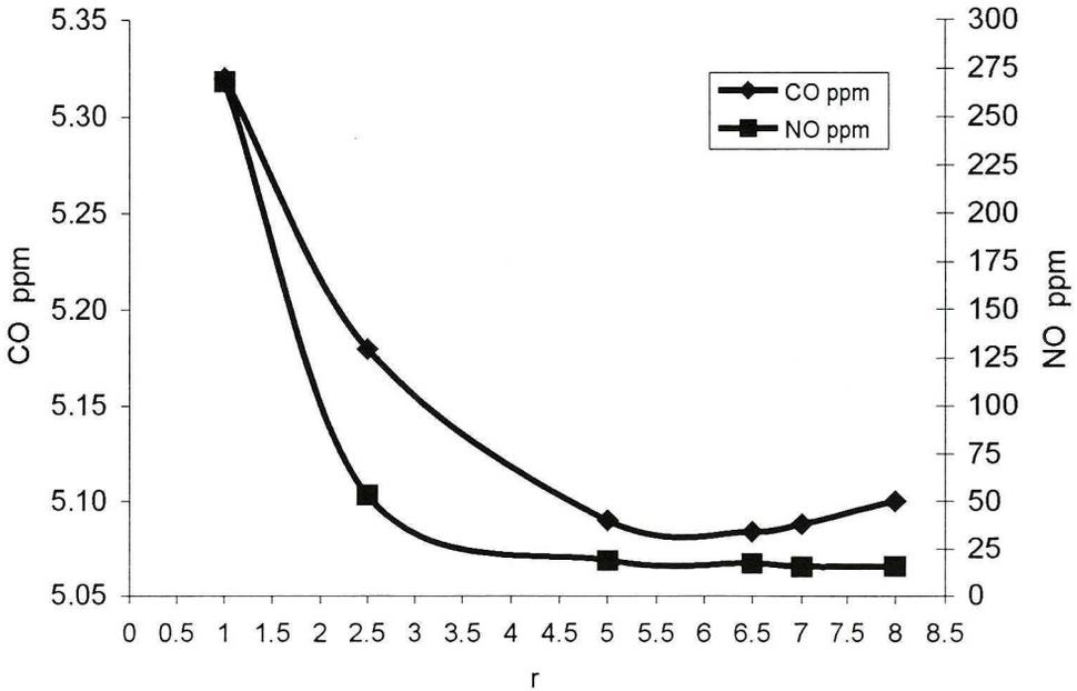
Fig. 8. Calculated final CO and NO concentrations as functions of recirculation rate  $r$  for air temperature 1350K
