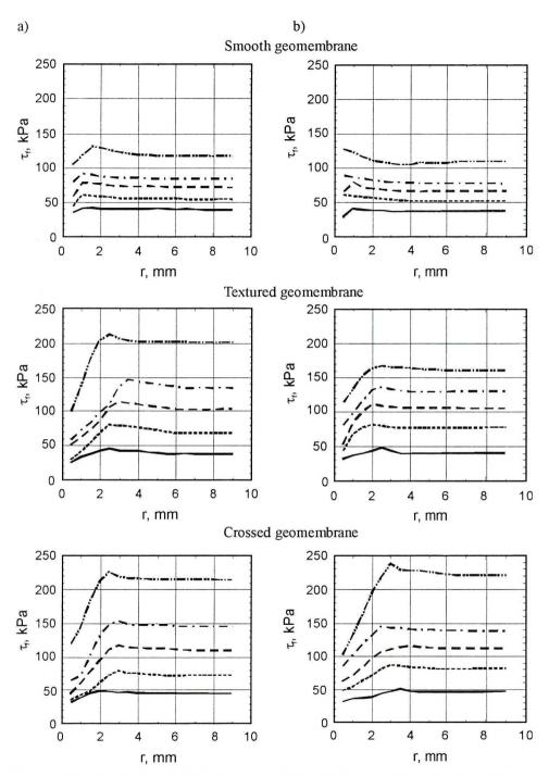
Fig. 5. Relationship graphs of fly ash/bottom ash mix – HDPE geomembrane shear strength in dependence on sample displacement r, tested at values of normal stress  $\sigma$  equalled 50, 100, 150, 200 and 300 kPa, for samples compacted by Standard or Modified Proctor method: a) standard mix compaction, b) modified compaction
