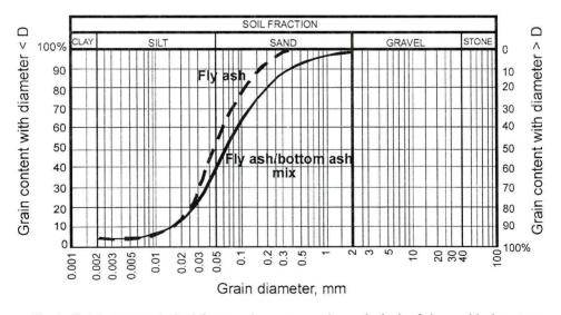
Fig. 1. Graining curves obtained for averaging waste samples on the basis of sieve and hydrometer analysis
