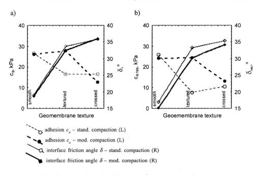
Fig. 8. Relationship between interaction friction angle  $\delta$  or adhesion  $c_a$  and tested geomembrane texture: a) peak parameters, b) residual parameters
