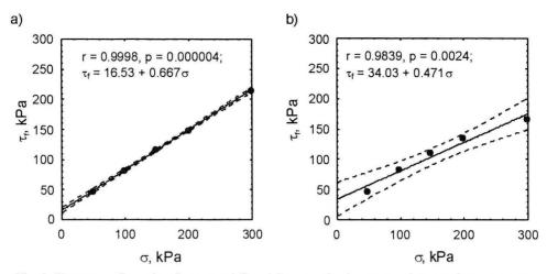
Fig. 6. Shear strength graphs of compacted fly ash/bottom ash mix – textured geomembrane contact: a) standard mix compaction, b) modified compaction
