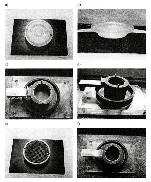
Fig. 4. Cylindrical box of direct shear apparatus with additional instrumentation: a) top view of PC platen for geomembrane, b) PC platen fixed in lower frame of apparatus box – end view, c) cylindrical box with PC platen – top view, d) end view of box, e) PC platen with crossed geomembrane, f) top view of box with geomembrane
