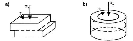
Fig. 2. Shearing scheme in direct shear apparatus: a) classical-box, b) torsional-ring
