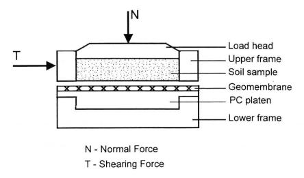
Fig. 3. Scheme of direct shear apparatus modified for interface contact tests
