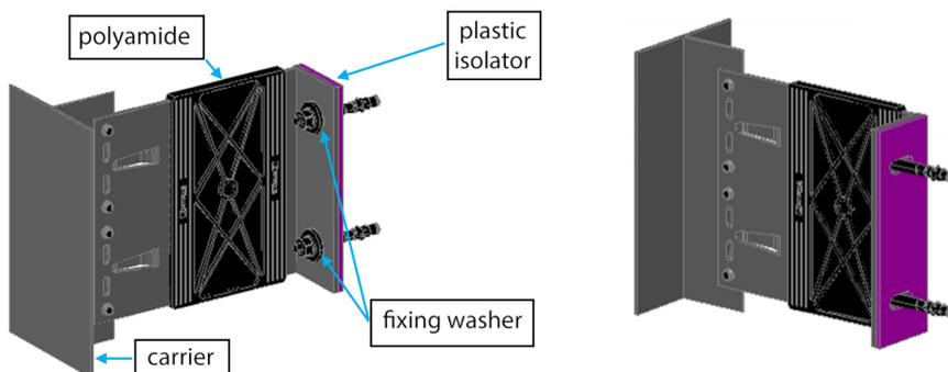
Fig. 2. Aluminium brackets with polyamide thermal break overview
