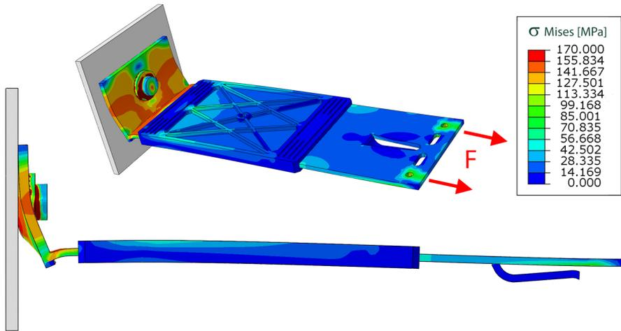
Fig. 7. The deformation mode and stress distribution pattern during the tension test
