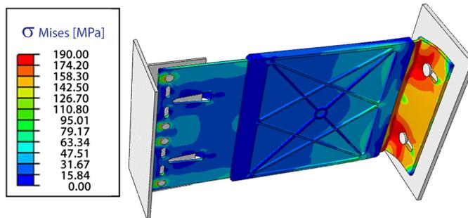
Fig. 11. Stress concentration points at the fixing holes, prying effect
