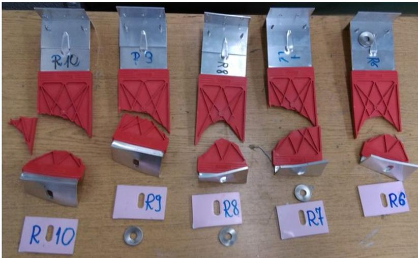
Fig. 15. Testing the plastic/ aluminium joint strength
