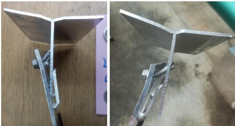
Fig. 13. Failure of brackets by pulling out the screws securing the curtain wall backup structure
