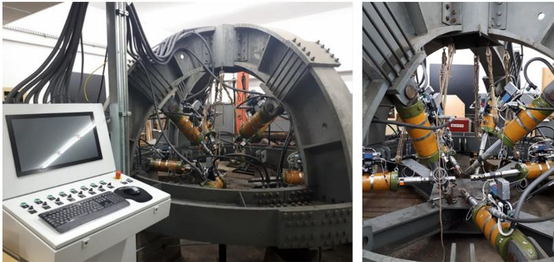
Fig. 4. Test stand for multi-directional strength testing
