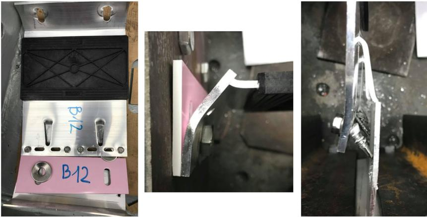
Fig. 10. Failure modes of helping hand brackets
