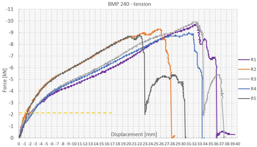
Fig. 6. Graphical representation of the results of testing the BMP 240 bracket under tensile force
