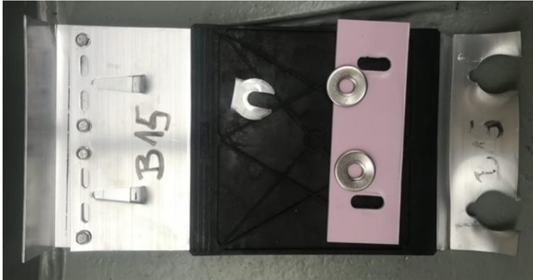
Fig. 12. Final failure – bracket pulled apart at the weakened point of aluminium foot
