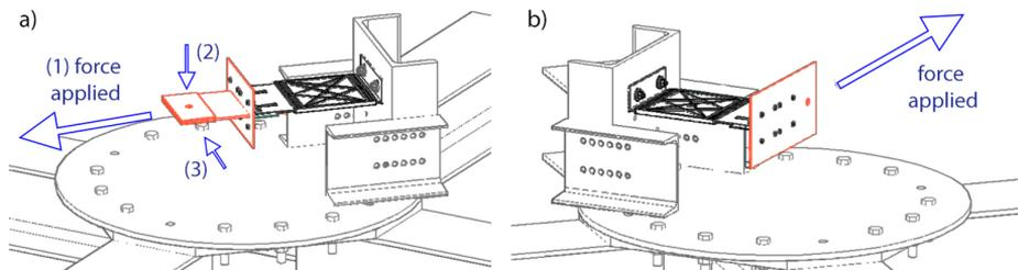
Fig. 5. Bracket mounting and loading setup on multi-directional strength test stand
