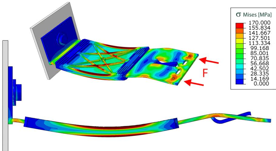
Fig. 8. Deformation mode and stress distribution pattern during the compression test
