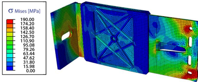
Fig. 14. Hanger failure model. Stress concentration points at the backup frame stud fixing holes
