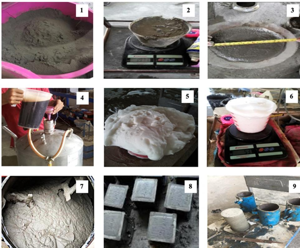
Fig. 2. Process flow of making FC
