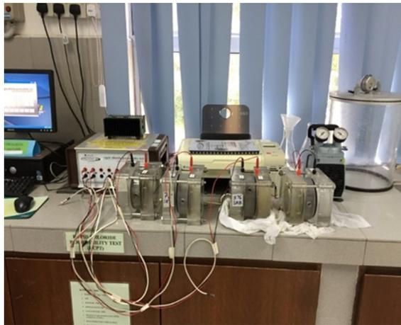
Fig. 4. Rapid Chloride Permeability Test set up
