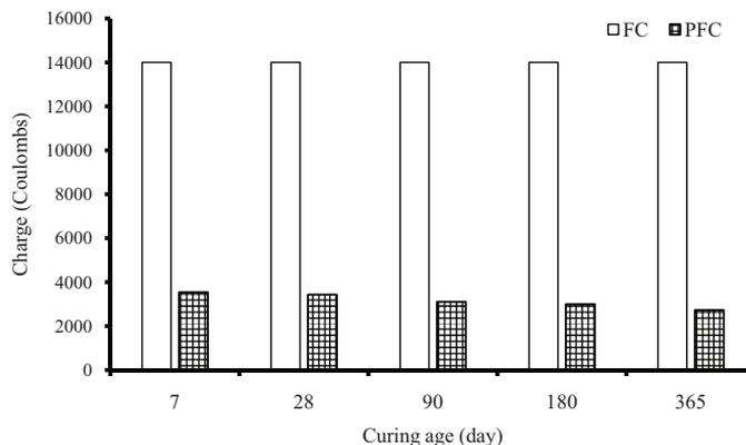
Fig. 11. Rapid chloride permeability of FC and PFC
