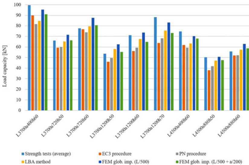
Fig. 8. Load capacities obtained by various methods
