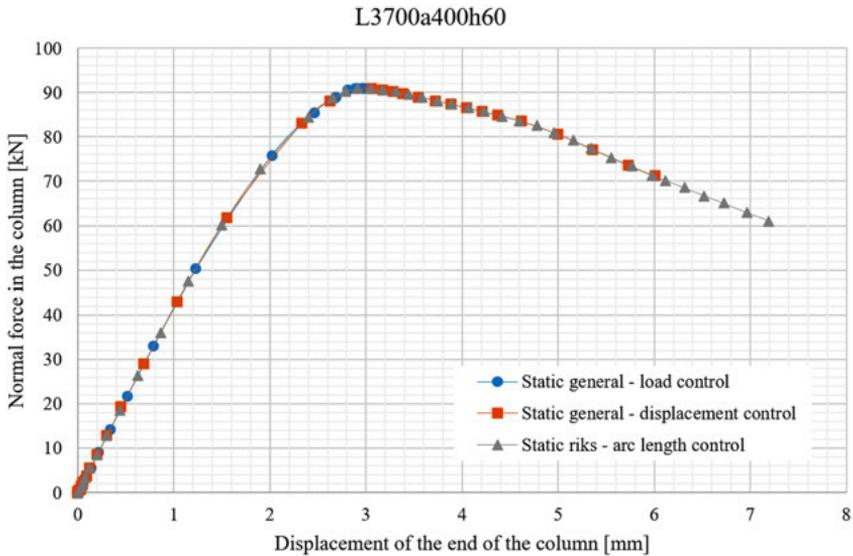
Fig. 3. The force-displacement graph for  $L3700\ a400\ h60$
