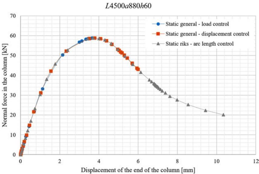
Fig. 4. The force-displacement graph for  $L4500\ a880\ h60$
