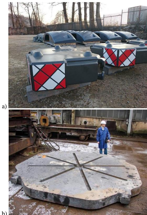
Fig. 1. Examples of counterweight (a) and bottom plates (b) produced in Foundry Krakodlew S.A.
