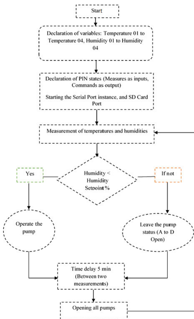
Fig. 2. Flowchart for temperature measurement and soil moisture control; source: own elaboration
