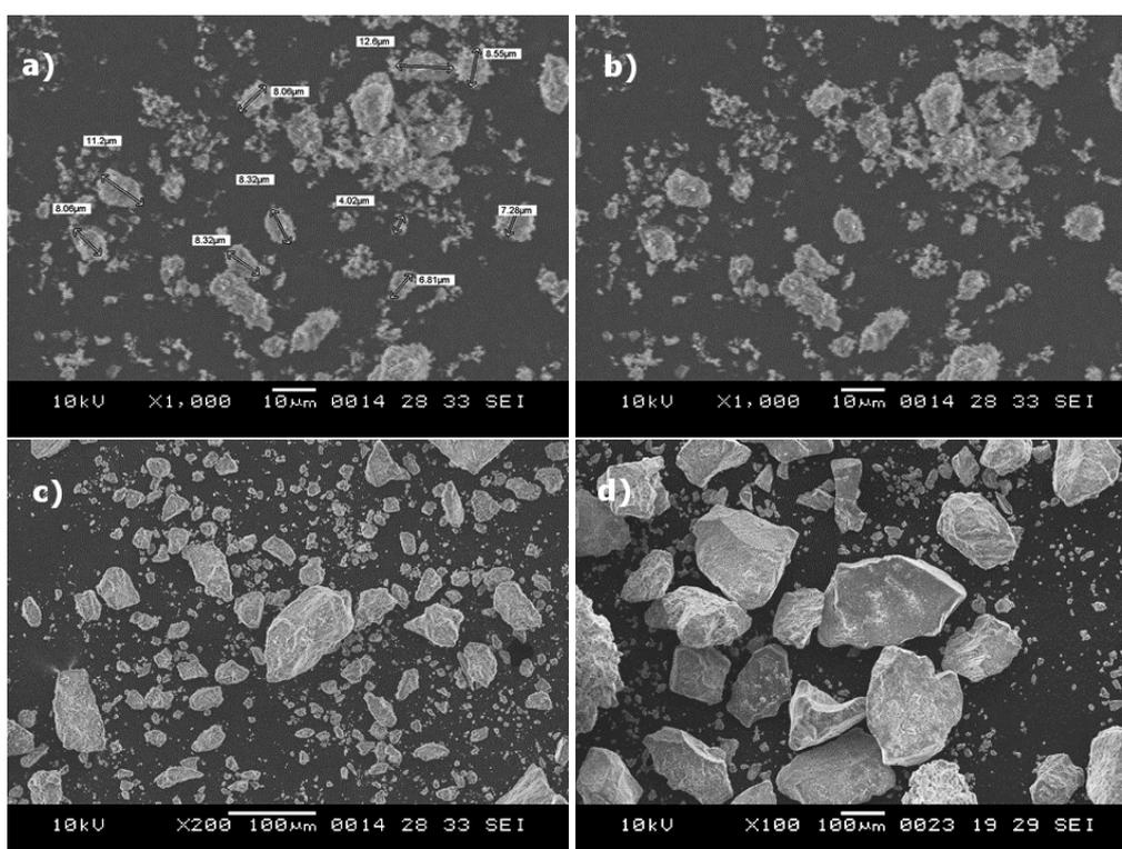
Fig. 4. SEM micrographs of synthesized (a) UEGA<sub>90</sub>, (b) UEGA<sub>70</sub>, (c) UEGA<sub>50</sub>, (d) EGA
