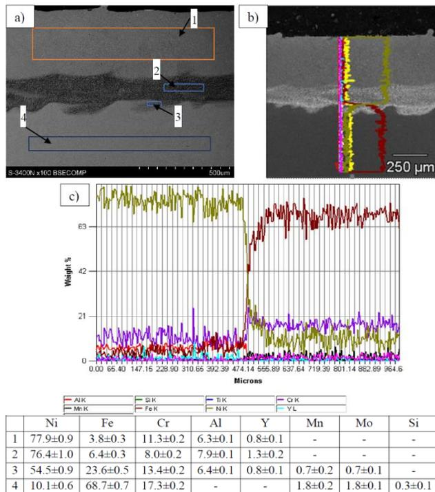
Fig. 2. The chemical composition of as-clad NiCrAlY coating on 316L steel (in wt %)
