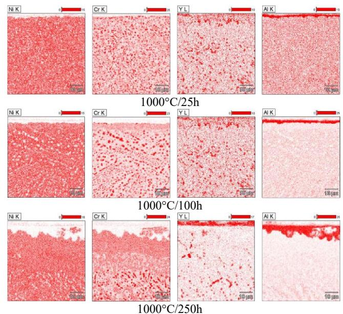
Fig. 9. Microstructure of NiCrAlY coating on 316L alloy after annealing at 1000°C/10-250h – alloying elements distributions
