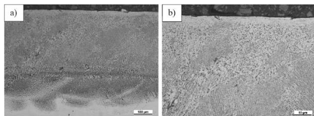
Fig. 3. Microstructure of NiCrAlY coating on 316L alloy after annealing at 1000°C/25h
