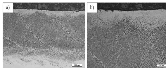
Fig. 5. Microstructure of NiCrAlY coating on 316L alloy after annealing at 1000°C/100h
