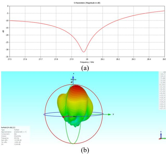
Fig. 9. Simulation results for  $2 \times 2$  circular patch antenna array with optimum element spacing  $dy = 0.6128\lambda$  and spacing  $dx = 0.85\lambda$ , (a) return loss  $S_{11}$  (b) 3D-radiation pattern
