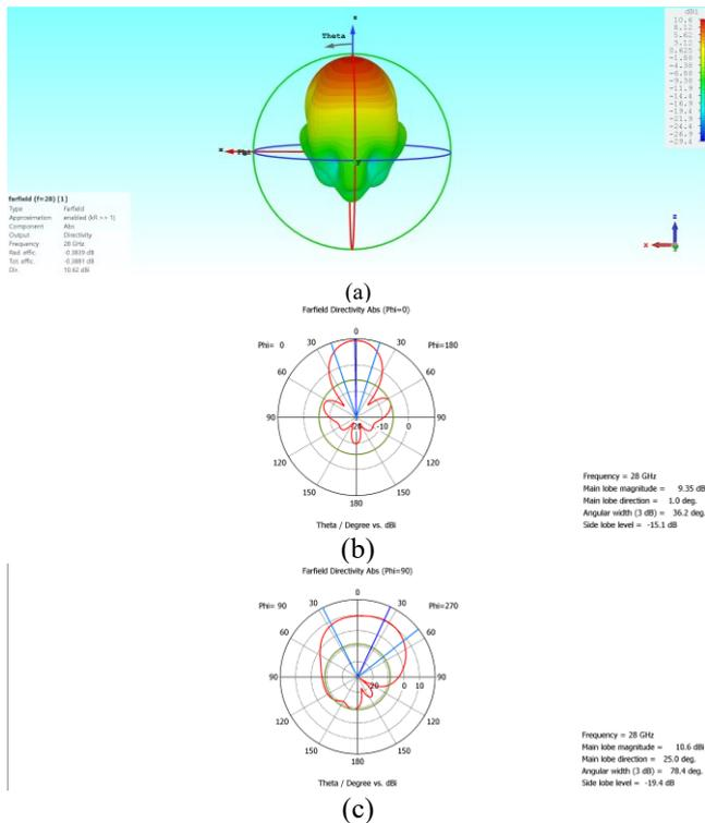
Fig.7. Simulated radiation patterns at 28 GHz of 1 x 2 circular patch antenna array for optimum element spacing  $0.6128\lambda$  (a) 3D (b) 2D in E-plane (c) 2D in H-plane.
