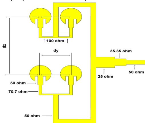
Fig. 8. Geometry of 2 x 2 circular patch antenna array
