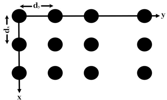
Fig. A.1. M × N planer patch antenna array configuration in xy plane
