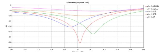
Fig. 6. Comparison of Return loss  $S_{11}$  for  $1 \times 2$  circular patch antenna array with particular element spacing's ( $0.5\lambda$ ,  $0.55\lambda$ ,  $0.6\lambda$ ,  $0.625\lambda$ ,  $0.65\lambda$ )
