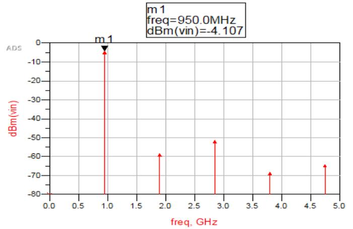
Fig. 4. input power without matching with GSM 900 downlink frequency input of -10dbm source
