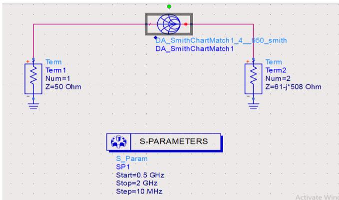
Fig. 13. Smith chart connection in ADS for impedance matching with GSM 900 downlink frequency input of -10dbm source
