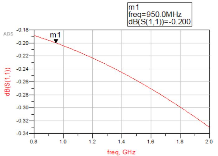
Fig. 6. reflection coefficient ( $S_{11}$ ) before matching with GSM 900 downlink frequency input of -10dbm source
