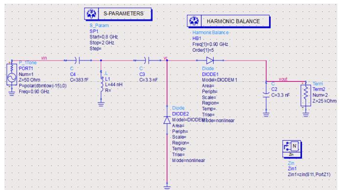
Fig. 21. Energy harvesting circuit design after including the designed matching circuit with GSM 900 uplink frequency input of -10dbm source
