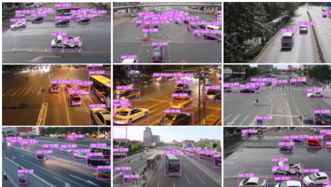
Fig. 8. Detection examples of Mob_YOLOv5 in different scenarios
