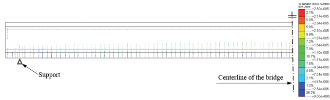
(a) Semi-elevation view of cracks
