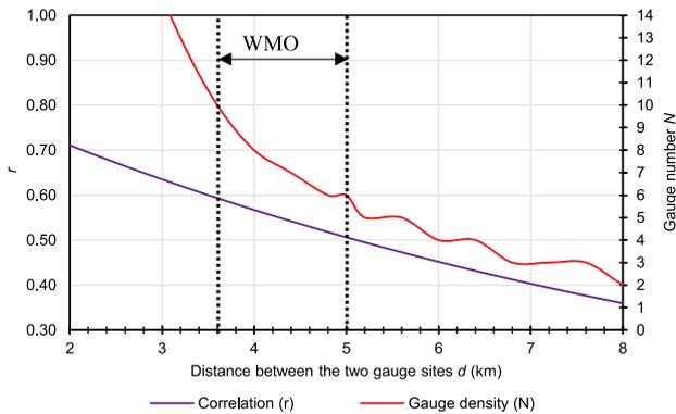
Fig. 12. Gauge density and correlation vs. gauge distance; source: own study
