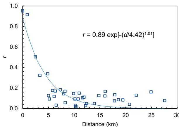
Fig. 9. Intergauge correlations (squares) and the fitted exponential function (curve) for 30-min time averaging;  $r$  = correlation coefficient,  $RMSE$  = root mean square error,  $d$  = distance between the two gauge sites; source: own study
