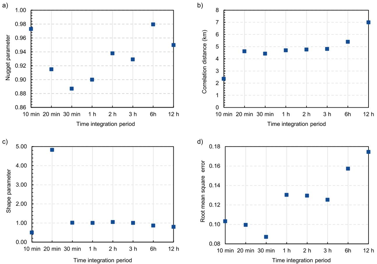
**Fig. 10.** Dependence of: a) nugget parameter, b) correlation distance, c) shape parameter of the exponential function, d) root mean square error (RMSE), on the averaging time scale ranging from 10 min to 12 h; source: own study
