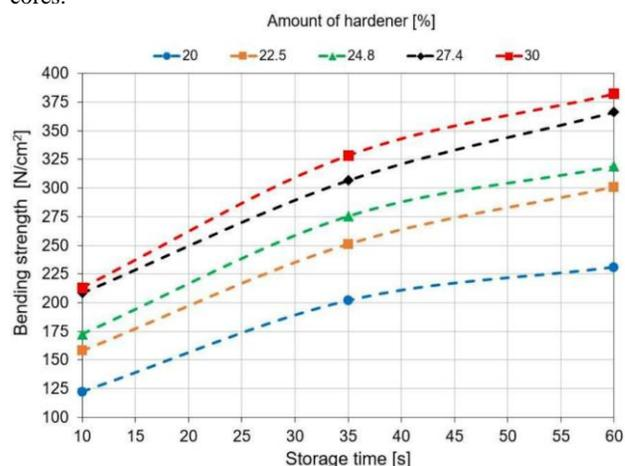
Fig. 3. The hardening characteristic of the warm-box sand specimens after removing from the core-box up to 60 s
