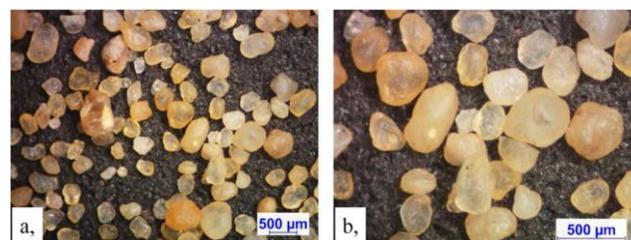
Fig. 1. Stereomicroscopic image of the reclaimed sand grains at a magnification of 20x (a) and 40x (b)
