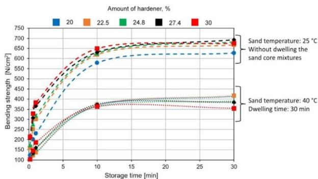
Fig. 7. The combined effect of the increased sand temperature and dwelling time on the hardening characteristic of the warm-box sand cores
