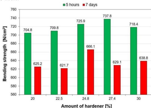
Fig. 5. Storage ability of the warm-box bending test bars
