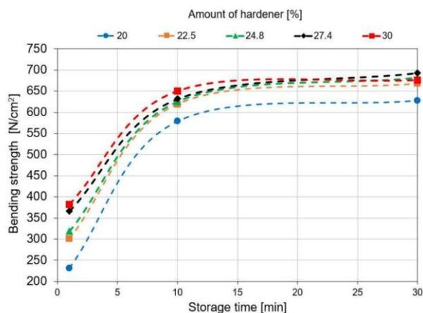
Fig. 4. Hardening characteristic of warm-box sand specimens from 10 minutes to 30 minutes of storage time
