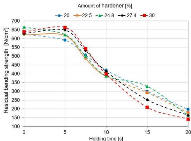
Fig. 6. Residual bending strength of sand specimens after thermal exposure
