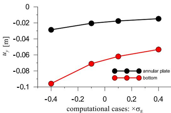
**Fig. 4.** The relationship – deflections vs variable subsoil stiffness
