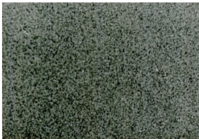
Fig. 11. Macrostructure of upper surface of continuous cast strip (x10)
