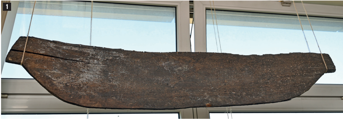
Fig. 1 A specimen of archeological wood – a "black oak" floorboard from a house in Elbląg; first half of the thirteenth century (reclaimed wood)
