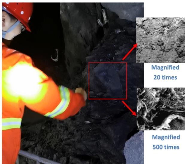
Fig. 4. Collection of soft rock samples in underground mines
