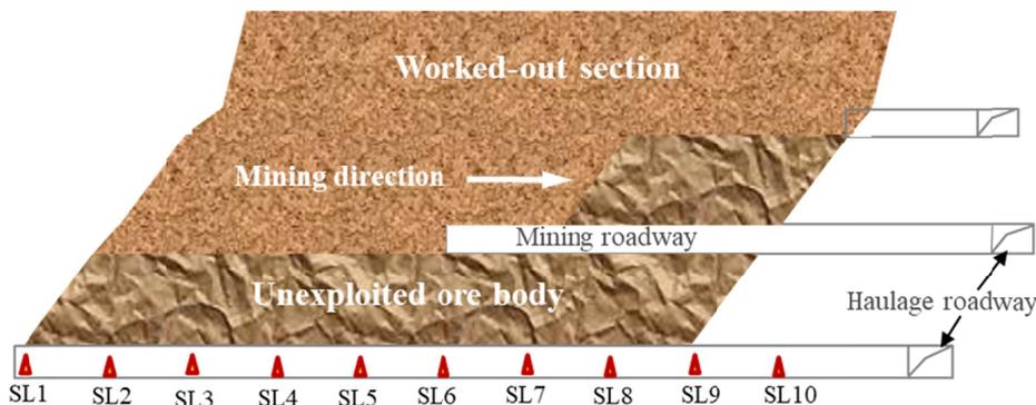
Fig. 8. Layout plan of Mine-TCS monitoring equipment
