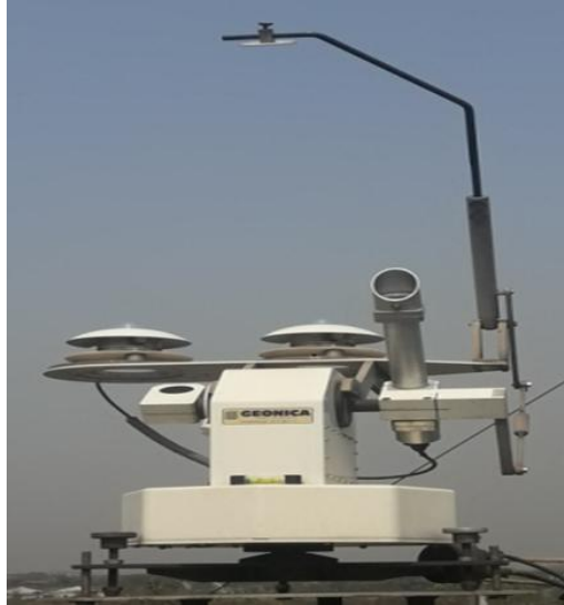
Figure 10: Photograph of digital pyranometer system.
