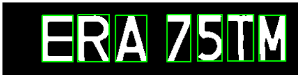
Fig. 3. Character segmentation. Individual characters are marked with a green frame.
