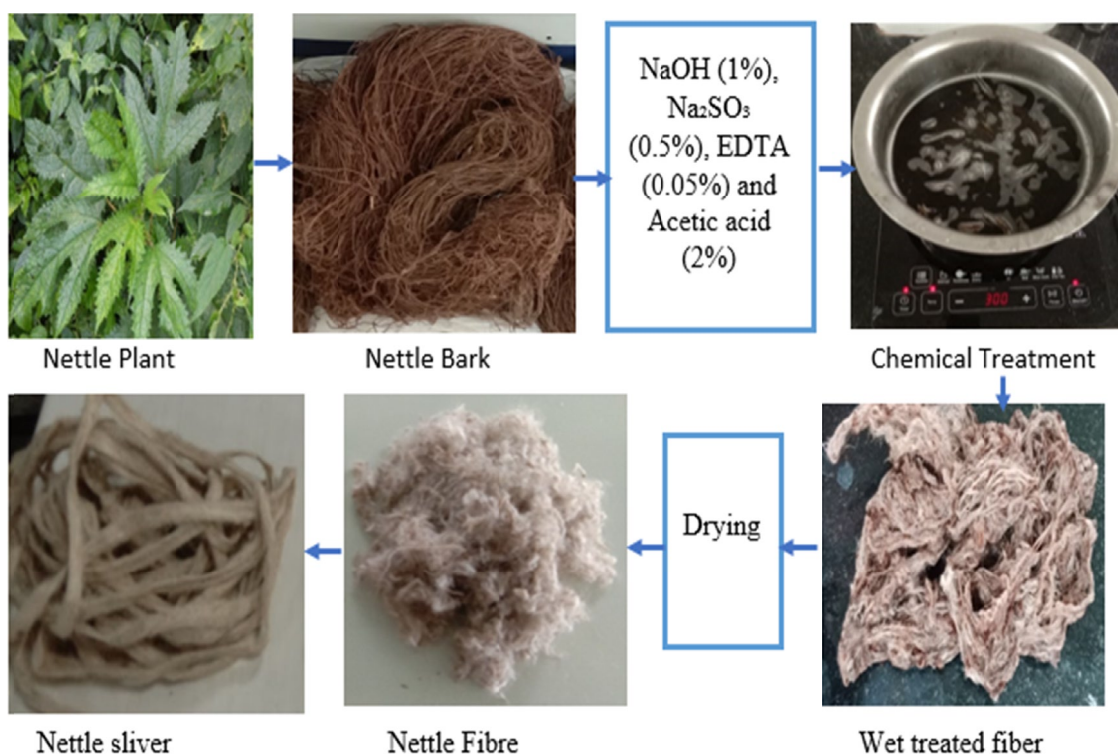
Fig. 2. Chemical treatment process on nettle fibre
