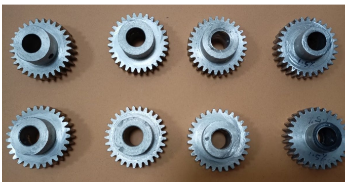
Fig. 4. Manufactured Al-nano \text{Al}_2\text{O}_3 composite spur gears
