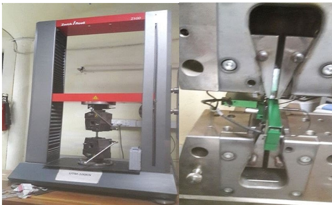
Fig. 7. Machine setup for Tensile testing
