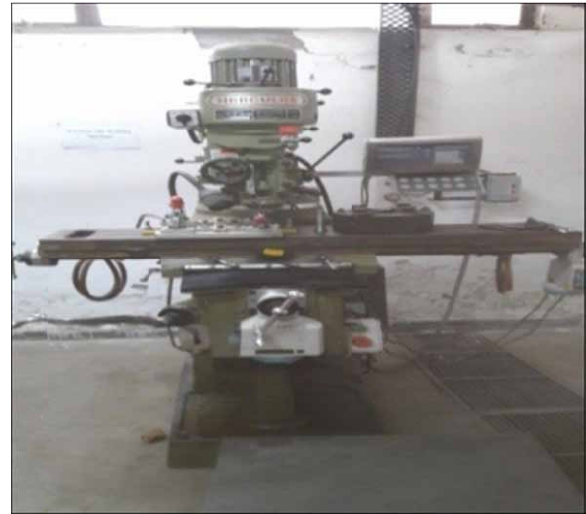
Fig. 1. Vertical Milling Machine (Hercules) for FSW Process
