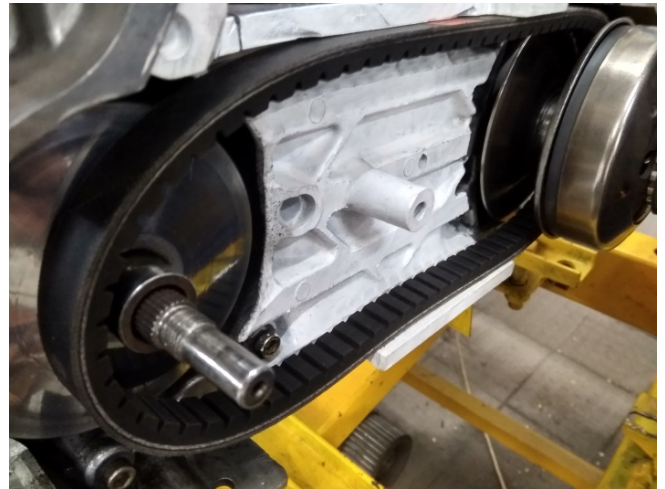
Fig. 7. Body of CVT gear prepared for recording footage
