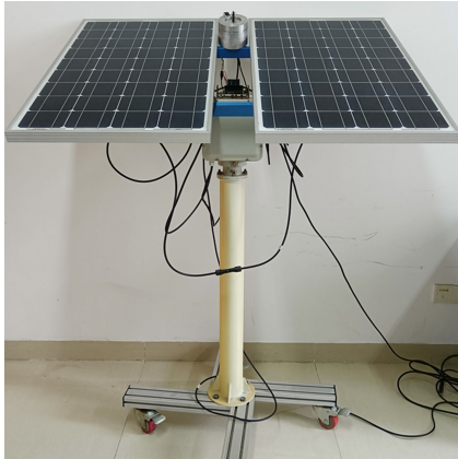
a) Two-axle sun tracking experimental facility.
