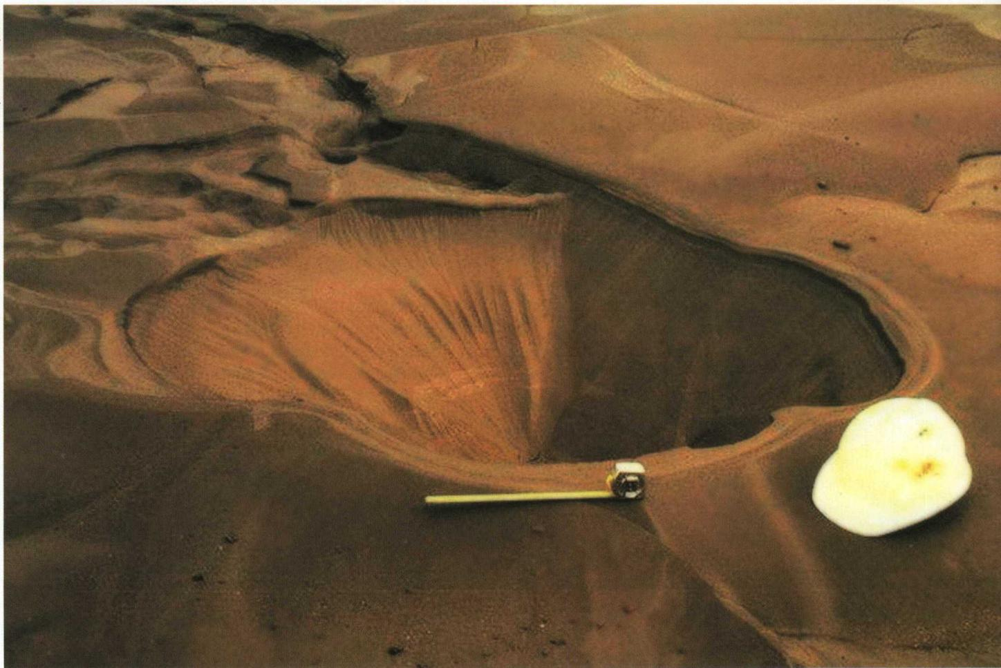
Surface craters indicate the appearance of the sudden dissipation of pore pressure, in the form of geysers of a water-soil mixture
