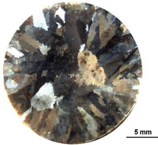
Fig.2 . Macrostructure of CuSi3Zn3FeMn1 alloy in sand casting
