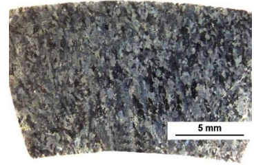
Fig. 4. Macrostructure of CuSi3Zn3FeMn1 alloy from fragment of sleeve in centrifugal casting
