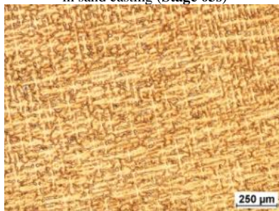
Fig. 12. Microstructure of CuSi3Zn3FeMn1Ni1.8 alloy of gravity die casting (Stage 03d)
