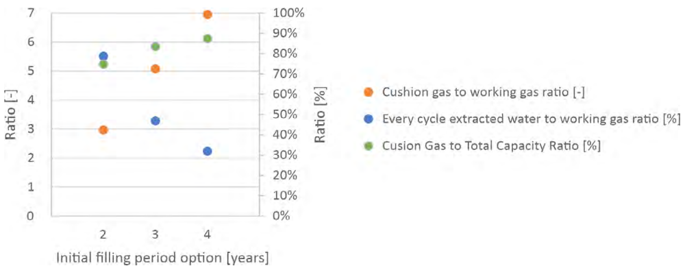
Fig. 7. Graph showing the comparison of ratios: every cycle extracted water to working gas, cushion gas to total capacity and cushion gas to working gas
