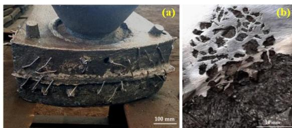
Fig. 1. Casting with visible reinforcement zone: (a) from the front, (b) fragment perpendicular to the reinforcement axis (cut and broken)
