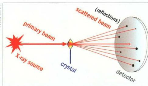
**A small crystal scatters the X-rays into a multitude of sharp reflections, the position and intensity of which are measured by electronic detectors**
