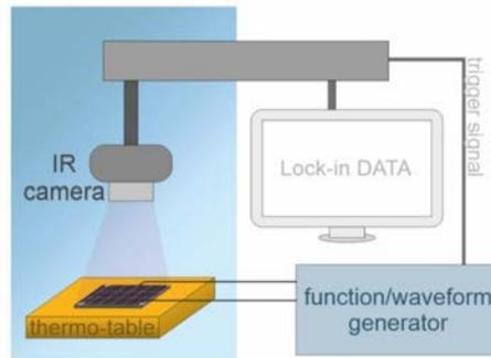
Fig. 10. Illustrative measurement system scheme of DLIT imaging.
