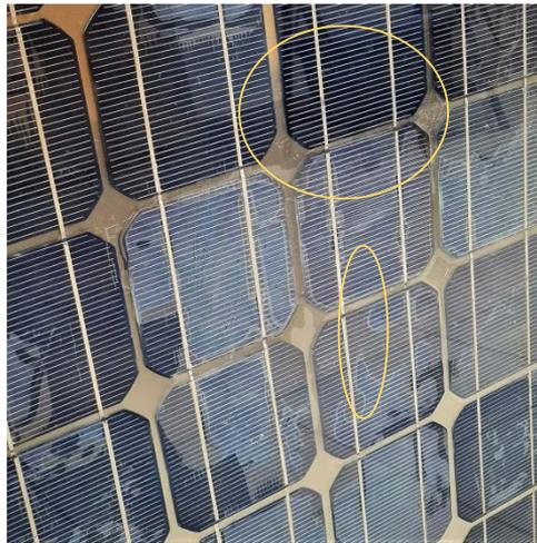
Fig. 2. Delamination of the photovoltaic panel on its surface.
