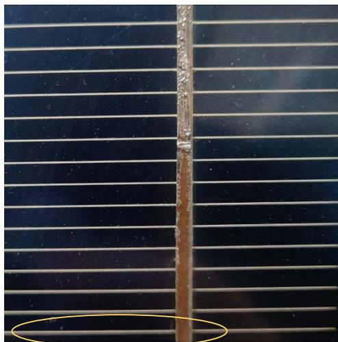
Fig. 5. Busbar degradation.
