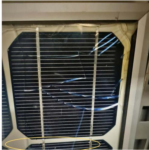
Fig. 4. Front glass breakages as a result of stress.
