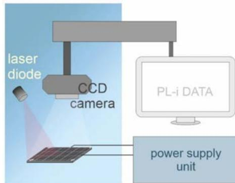
Fig. 7. Illustrative measurement system of the PL imaging.
