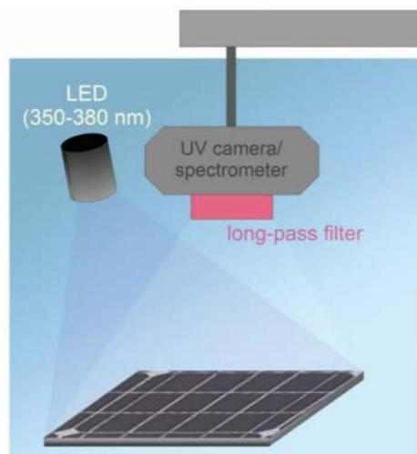
Fig. 9. Illustrative measurement system scheme of UV imaging.
