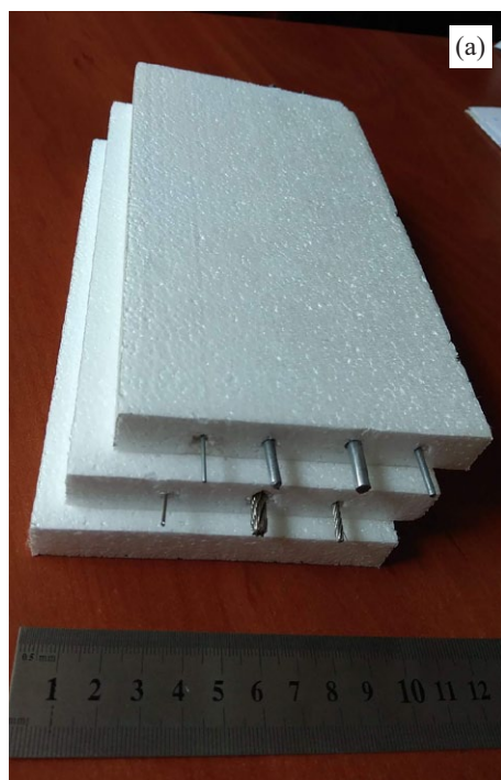
Fig. 1. EPS patterns with reinforcement (a) and castings (b)
