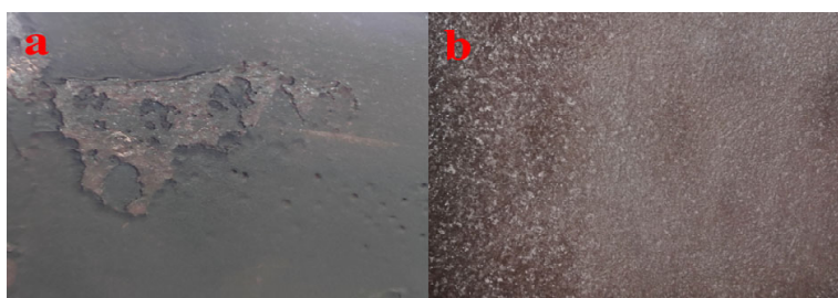
Fig. 5. Images of low arsenic anode passivation, 65°C, at current density of 250 A/m 2 (a) and normal anode dissolution, 65°C, at current density of 300 A/m 2 (b) respectively
