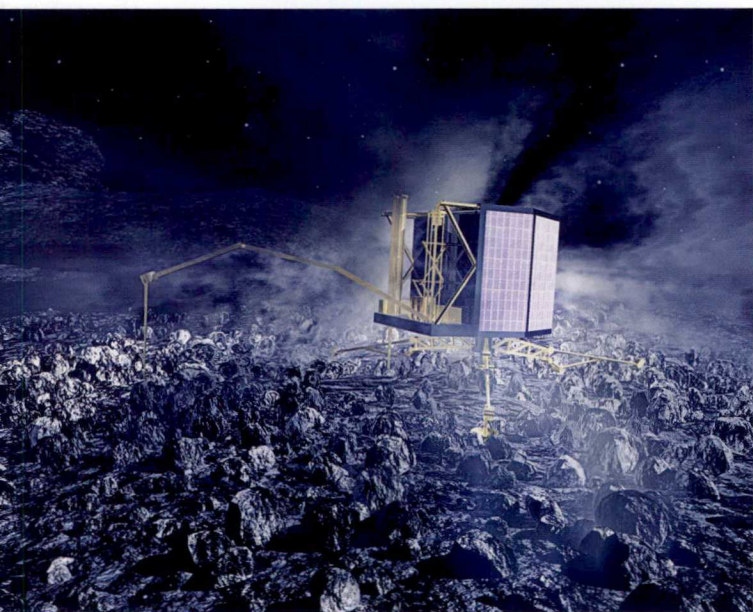
This artist's impression shows the Rosetta Lander anchored to the comet's surface with instruments, legs and solar panels
