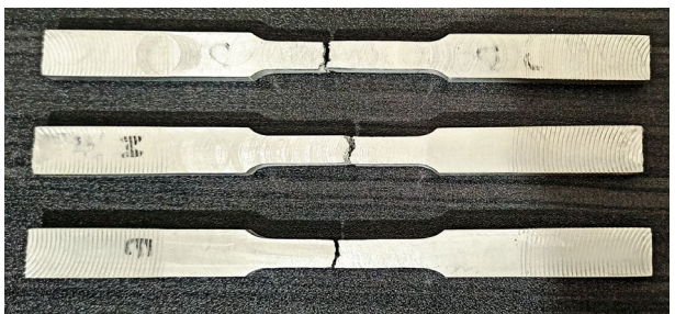
Fig. 9. (a) Tensile test of direct chill cast billets on the various positions along the cross-section of the billet diameter, (b) stress-strain diagram, (c) tensile test samples after fracture
