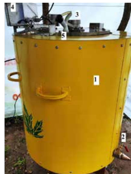
Figure 2. Pulsed air access batch bioreactor with the volume of working chamber 300 L: 1 – working chamber of the bioreactor; 2 – fitting for culture liquid sampling; 3 – special lock for air access; 4 – electronic fermentation control unit; 5 – fittings to introduce regulators.
