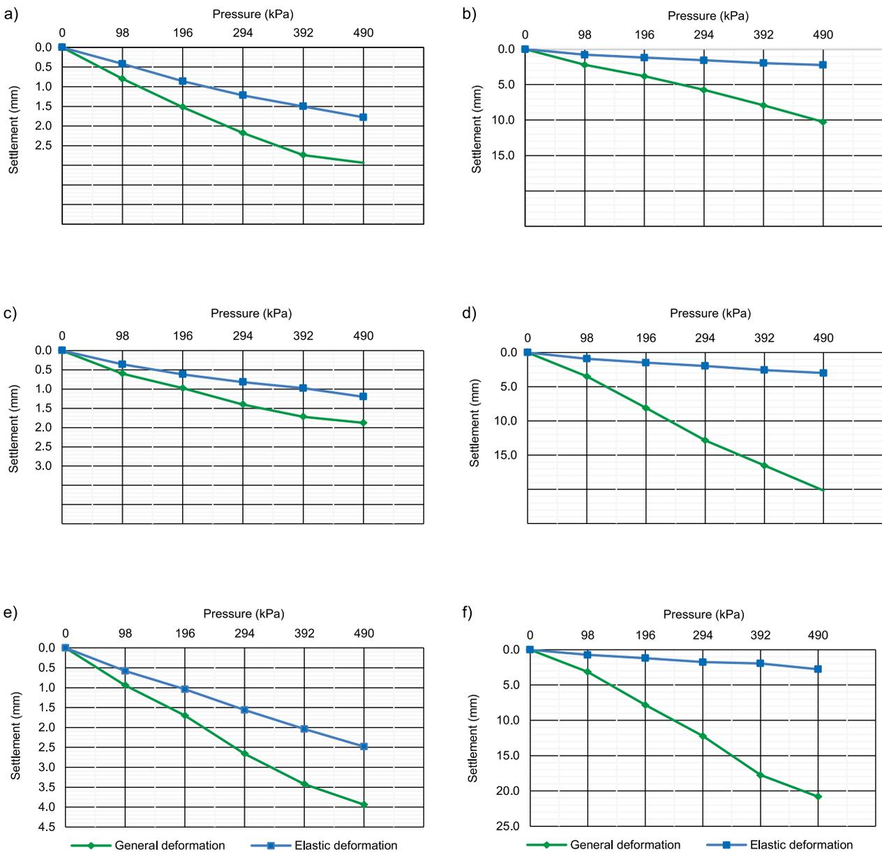
**Fig. 4.** Change of sample height and soaking: a) point 1 (dry soil), b) point 1.1 (wet soil), c) point 2 (dry soil), d) point 2.1 (wet soil), e) point 3 (dry soil), f) point 3.1 (dry soil); source: own elaboration
