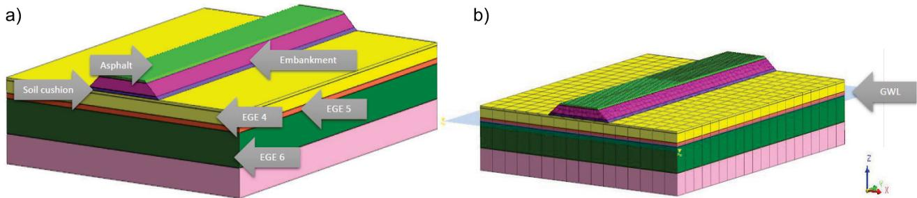
Fig. 3. Calculation model: a) with engineering-geological elements (EGE), b) with ground water level (GWL); EGE-4, EGE-5 and EGE 6 as in Tab. 3; source: own elaboration
