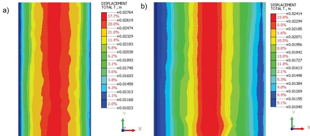
Fig. 7. General deformities: a) pavement, b) soil cushion; source: own study
