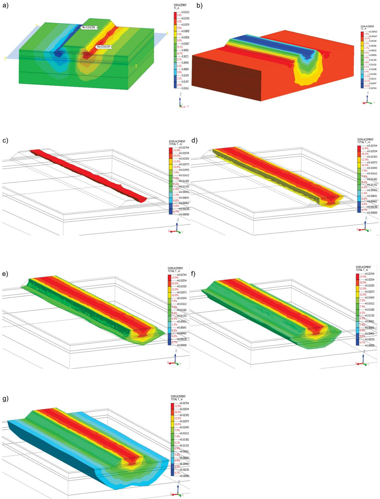
Fig. 6. Displacement of the embankment: a) x-axis, b) y-axis, c) at  $\geq 26$  mm, d) at  $\geq 20$  mm, e) at  $\geq 15$  mm, f) at  $\geq 10$  mm, g) at  $\geq 5$  mm; source: own study
