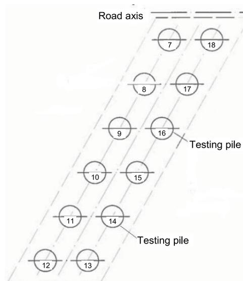
**Fig. 1.** Location of piles tested by static load; source: own elaboration
