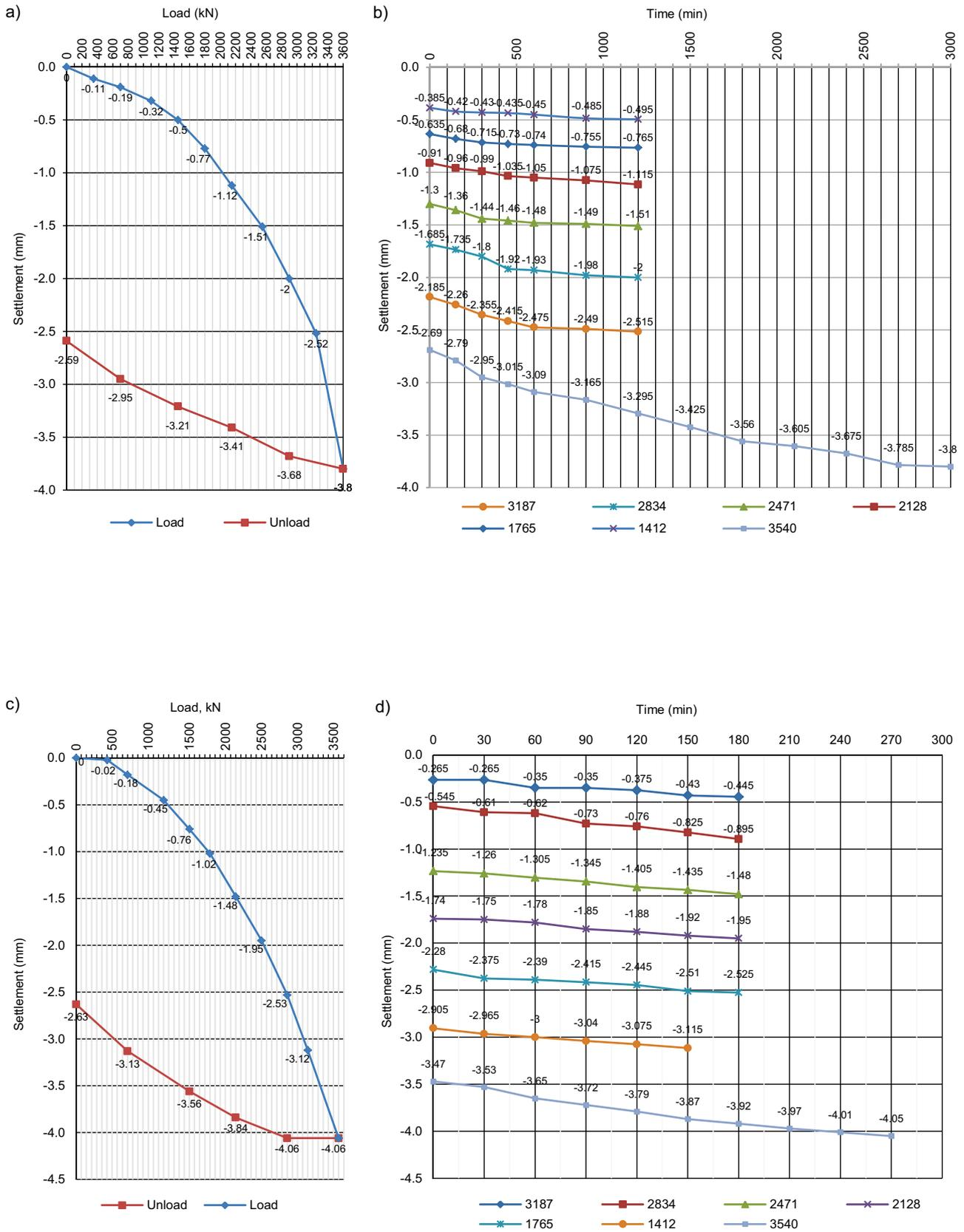
Fig. 5. Correlation of loading with settlement for pile 14: a) total settlement, b) by loading stages; for pile 16: c) total settlement, d) by loading stages; source: own study
