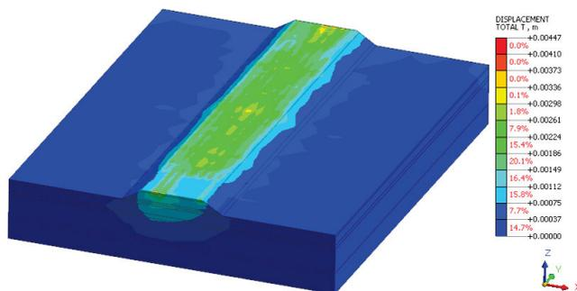
Fig. 8. Total embankment displacement due to road traffic; source: own study
