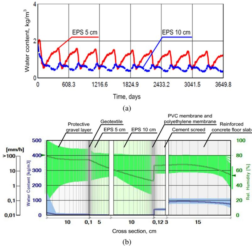
Fig. 5. Simulation of the partition's dampness change during ten years of use: a) water content in the layers of EPS, b) waveform of dampness change in the partition's layers
