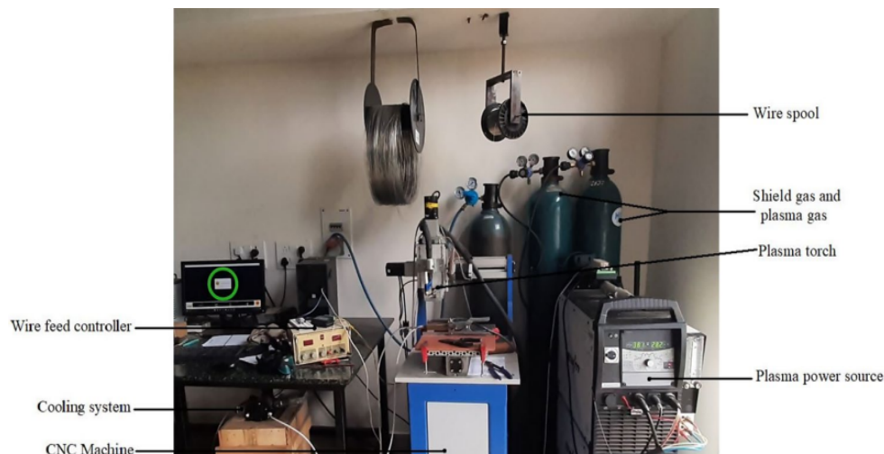
Fig. 1. Plasma beam remelting [15]
