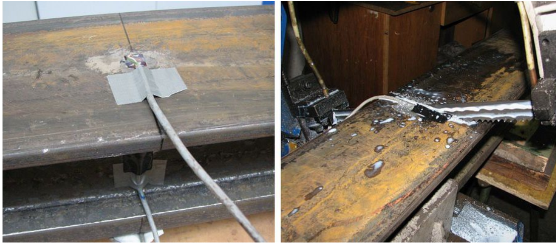
Fig. 3. Cutting method for tests on rail 60E1
