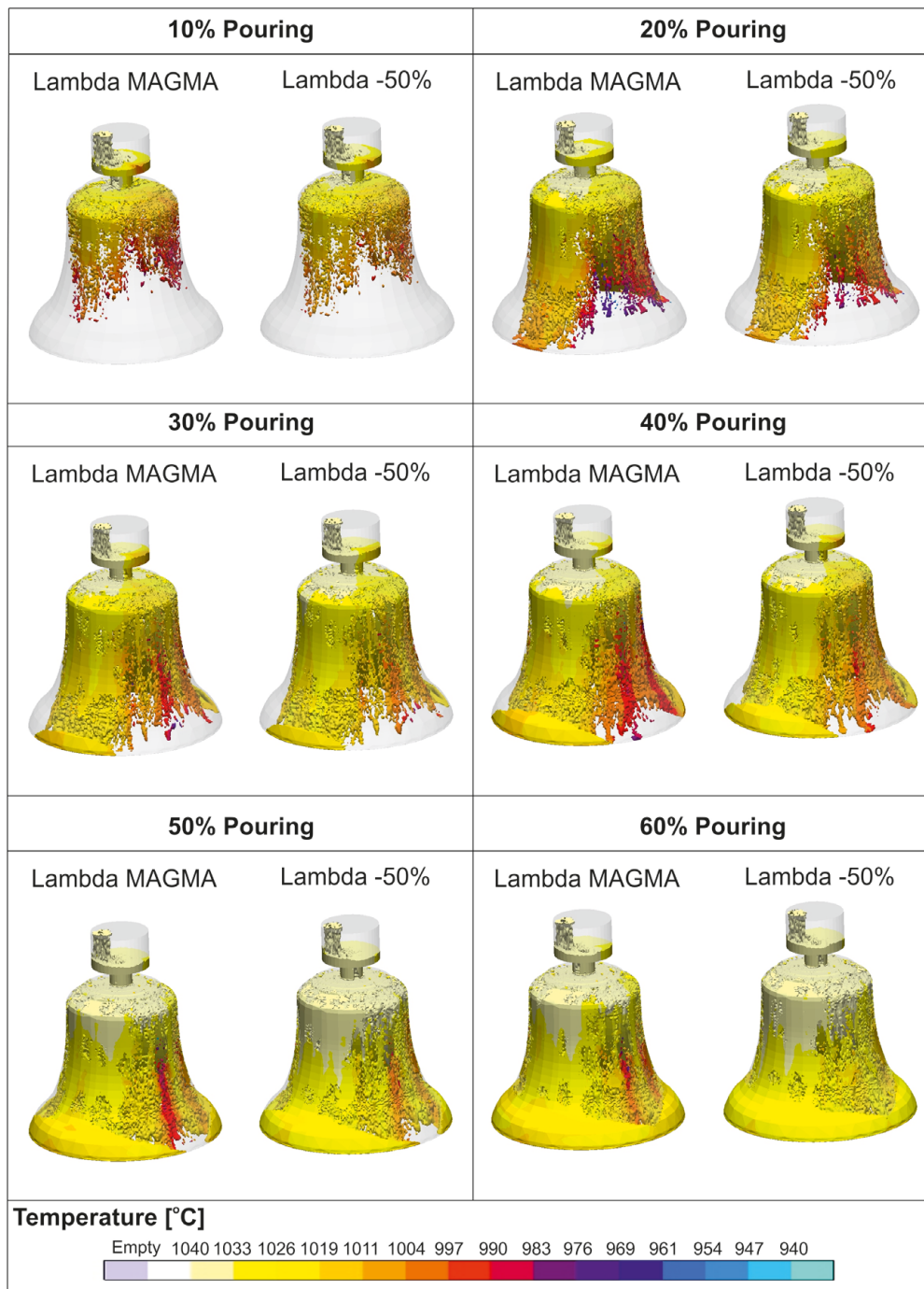
Fig. 5a. The distribution of the casting temperature when filling the mold cavity (pouring 10% to 60%)
