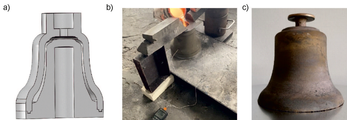
Fig. 1. The course of the experiment a) mold cross-section, b) mold during pouring, c) finished casting
