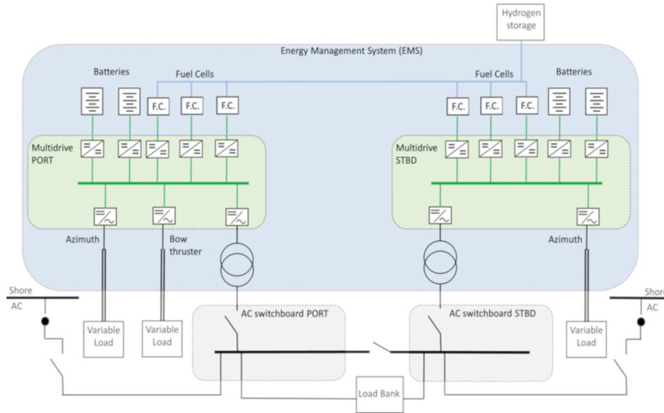
Figure 19: HySeas ferry propulsion system string test schematics [90].
