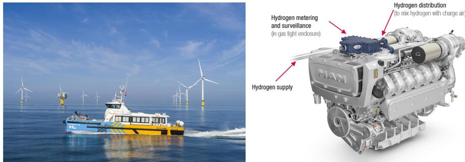
Figure 15: Hydrocat 48 [79] and MAN D2862 LE448 engine fitted to Hydrocat 48 [79].
