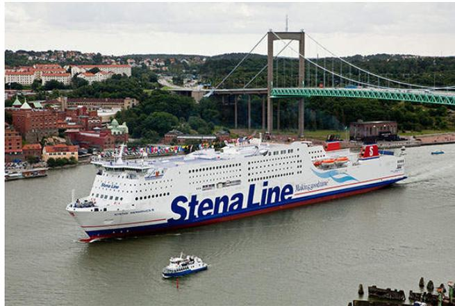
Figure 10: Stena Germanica – first commercial vessel to run on methanol [65].
