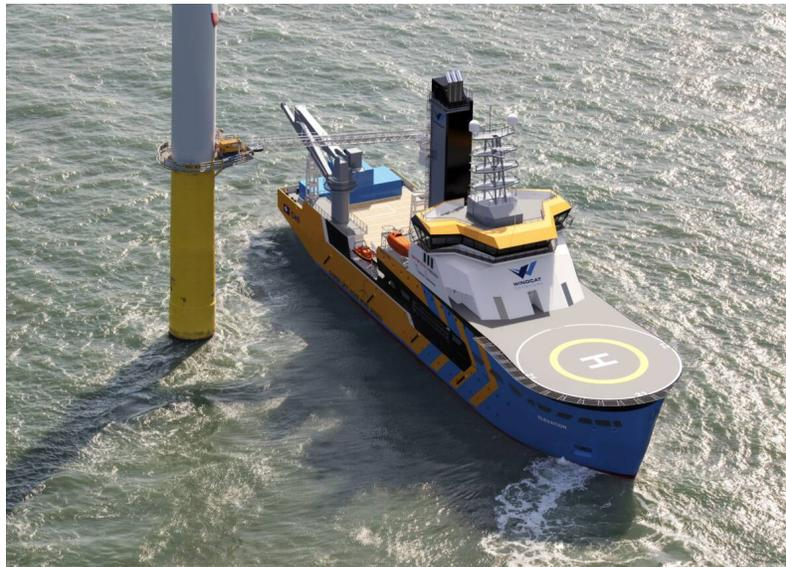
Figure 17: Windcat CSOV visualization [88].
