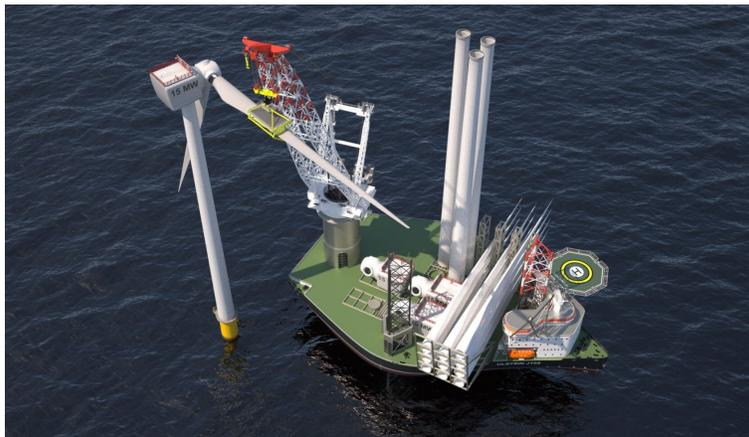
Figure 22: J102 wind turbine installation vessel – concept [94].
