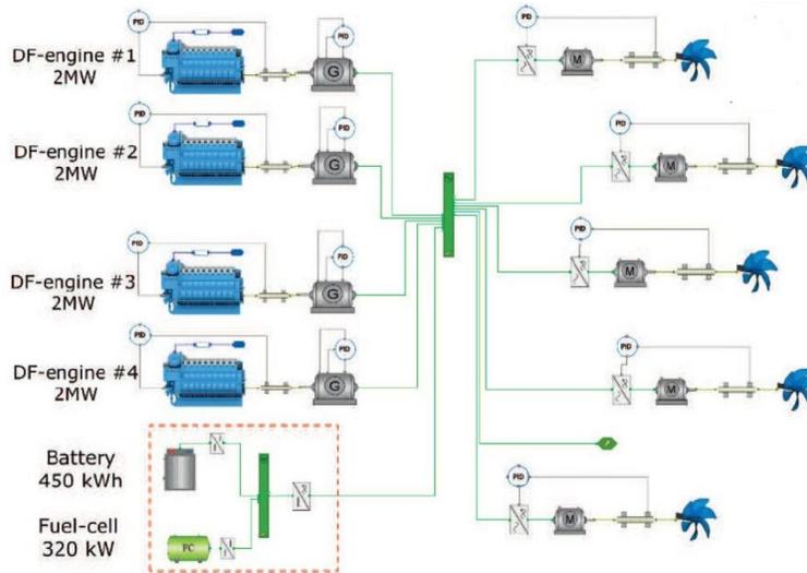
Figure 5: Battery – FC hybrid propulsion system on board the Viking Lady [55].
