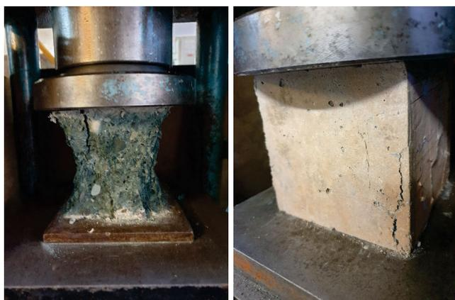
**Photo 1.** Illustrative representation of the study process carried out to explore the self-healing phenomenon in FRC specimens (phot.: A. Salmi)
