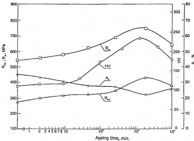
Fig. 8. Change of the mechanical properties with ageing time of CuNi10Al3 alloy with 0.4 wt % addition of Ti, homogenized at  $950^\circ\text{C}$ , water quenched and next aged at  $500^\circ\text{C}$
