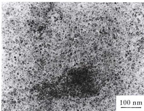
Fig. 22. Continuous precipitates of  $\gamma'$  phase in CuNi10Al3 alloy with 0.4 wt % addition of Nb, water quenched, deformed by  $\varepsilon = 40\%$ , aged at 500°C for  $2 \times 10^3$  minutes
