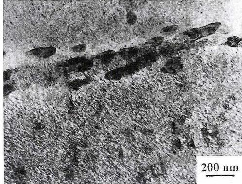
Fig. 3. Precipitates of  $\beta$  phase in CuNi10Al3 alloy with 0.4 wt % addition of Si, aged at 500°C for  $10^4$  minutes
