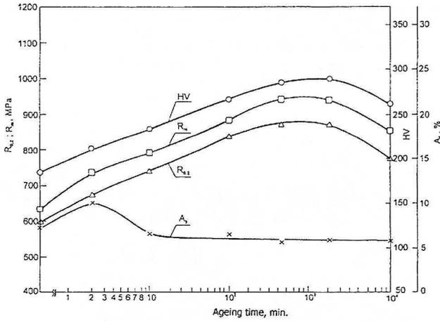
Fig. 11. Change of the mechanical properties with the ageing time of CuNi10Al3 alloy with 0.4 wt % addition of Ti, homogenized at 950°C, water quenched, deformed by  $\varepsilon = 40\%$  and next aged at 500°C
