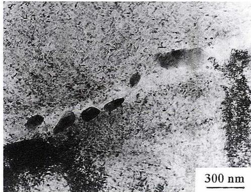
Fig. 7. Structure of CuNi10Al3 alloy with 0.4 wt % addition of Si, water quenched, deformed by  $\varepsilon = 40\%$  and next aged at  $500^\circ\text{C}$  for  $2 \times 10^3$  minutes
