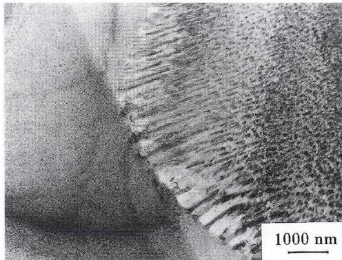
Fig. 16.  $\gamma'$  precipitates of discontinuous transition of CuNi10Al3 alloy with 0.4 wt % addition of Nb, aged at 500°C for  $10^4$  minutes
