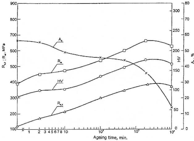
Fig. 15. Change of the mechanical properties with the ageing time of CuNi10Al3 alloy with 0.4 wt % addition of Nb, homogenized at 950°C, water quenched, and next aged at 500°C
