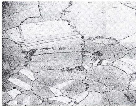
Fig. 18. Structure of CuNi10Al3 alloy with 0.4 wt % addition of Nb, aged at 500°C for  $10^4$  minutes. Magnified 250x
