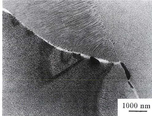
Fig. 17.  $\gamma'$  precipitates of continuous and discontinuous transition and  $\beta$  phase of CuNi10Al3 alloy with 0.4 wt % addition of Nb, aged at 500°C for  $10^4$  minutes
