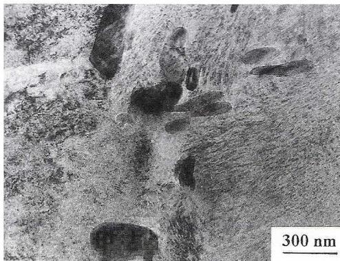
Fig. 20. Structure of CuNi10Al3 alloy with 0.4 wt % addition of Nb, supersaturated, deformed by  $\varepsilon = 40\%$  and aged at 500°C for  $2 \times 10^3$  minutes
