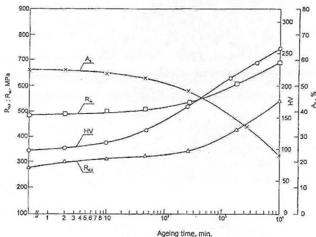
Fig. 1. Change of the mechanical properties with the ageing time of CuNi10Al3 alloy with 0.4 wt % addition of Si, homogenized at 950°C, water quenched and aged at 500°C
