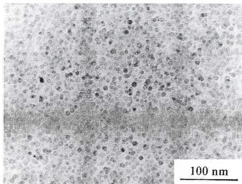
Fig. 9.  $\gamma'$  precipitates of continuous transition inside the grains of CuNi10Al3 alloy with 0.4 wt % addition of Ti, aged at  $500^\circ\text{C}$  for  $2 \times 10^3$  minutes
