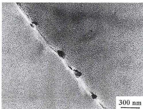
Fig. 10. Precipitates of  $\beta$  phase near the grain boundaries of CuNi10Al3 alloy with 0.4 wt % addition of Ti, aged at  $500^\circ\text{C}$  for  $2 \times 10^3$  minutes
