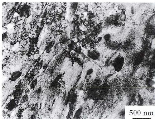
Fig. 21. Precipitates of  $\beta$  phase in the shear bands of CuNi10Al3 alloy with 0.4 wt % addition of Nb, water quenched, deformed by  $\varepsilon = 40\%$ , aged at 500°C for  $2 \times 10^3$  minutes
