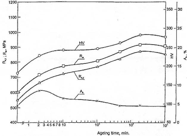
Fig. 5. Change of the mechanical properties with the ageing time of CuNi10Al3 alloy with 0.4 wt % addition of Si, homogenized at 950°C, water quenched, deformed by  $\epsilon = 40\%$  and aged at 500°C
