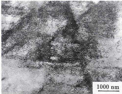
Fig. 12. Structure of CuNi10Al3 alloy with 0.4 wt % addition of Ti, water quenched, deformed by  $\varepsilon = 40\%$ , and next aged at 500°C for  $2 \times 10^3$  minutes
