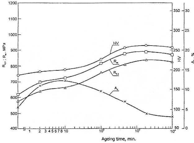
Fig. 19. Change of the mechanical properties of CuNi10Al3 alloy with 0.4 wt % addition of Nb, homogenized at 950°C, water quenched, deformed by  $\varepsilon = 40\%$  and aged at 500°C
