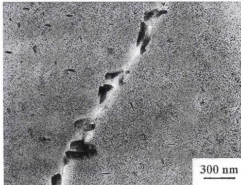
Fig. 4.  $Ni_3Si$  precipitates in grains and near the grain boundaries in CuNi10Al3 alloy with 0.4 wt % addition of Si, aged at 500°C for  $10^4$  minutes
