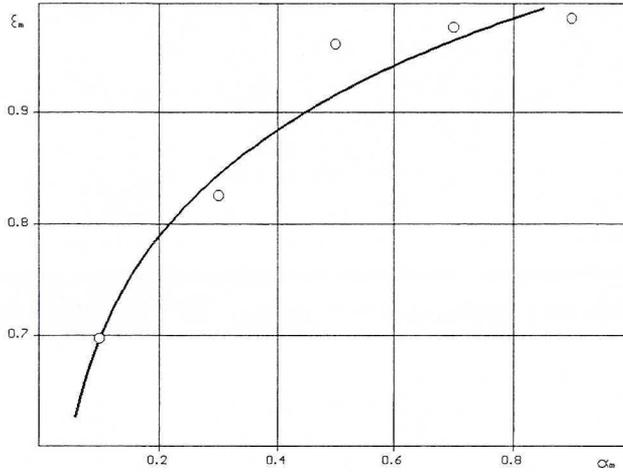
Fig. 1. Dependence of magnetic component recovery upon the content of this component in the feed
