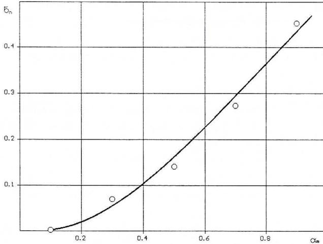
Fig.3. Dependence of non-magnetic component residue in the concentrate upon the content of magnetic component in the feed
