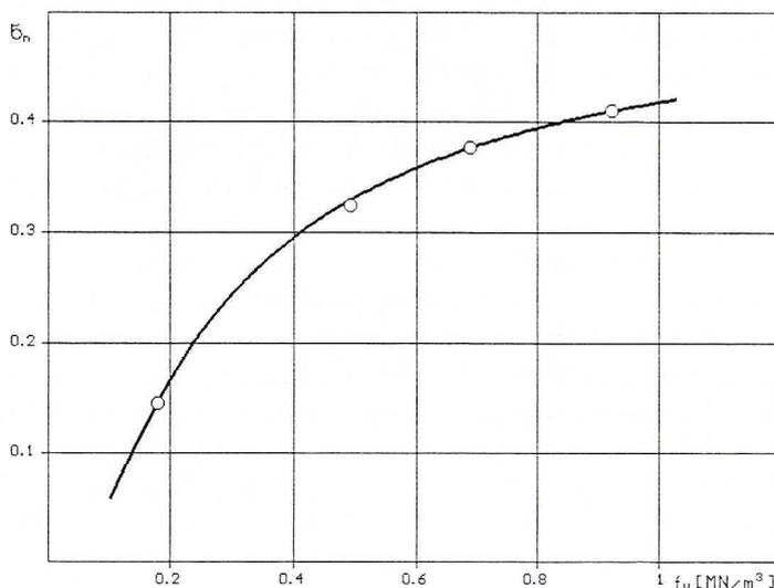
Fig. 4. Dependence of non-magnetic component residue in the concentrate upon magnetic force density
