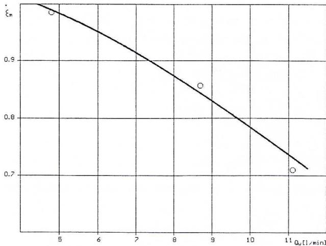
Fig. 2. Dependence of magnetic component recovery upon the amount of washing water
