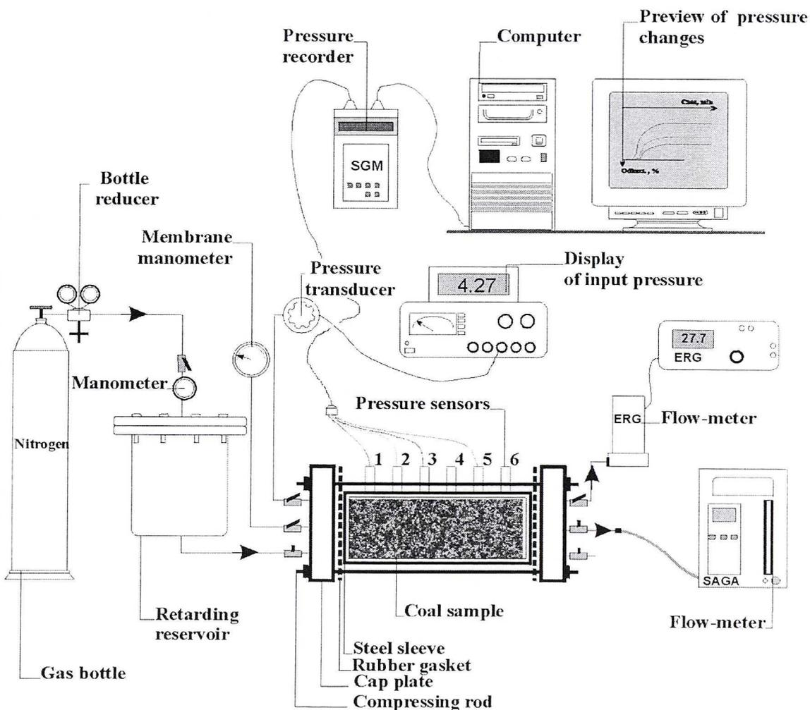
Fig. 1. The layout of the equipment for the flow investigations of gas flow
