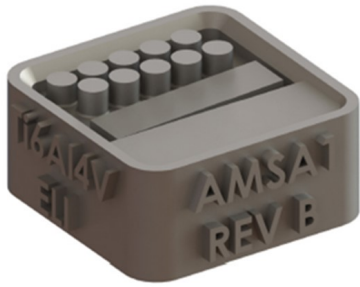
Fig. 21. Length artifacts: cylinders, angular surface, flat surface [9]
