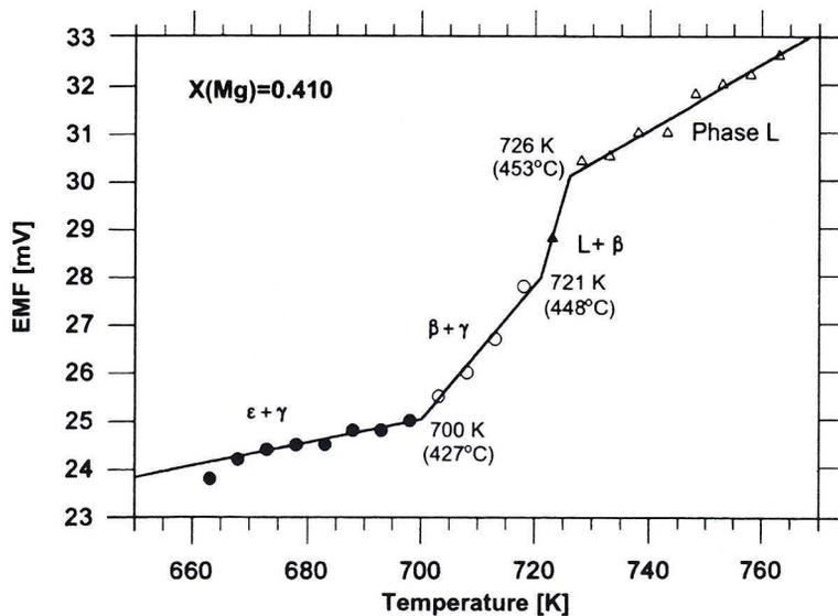
Fig. 3. Experimentally measured relation  $EMF = f[T]$  for concentration  $X(Mg) = 0.410$
