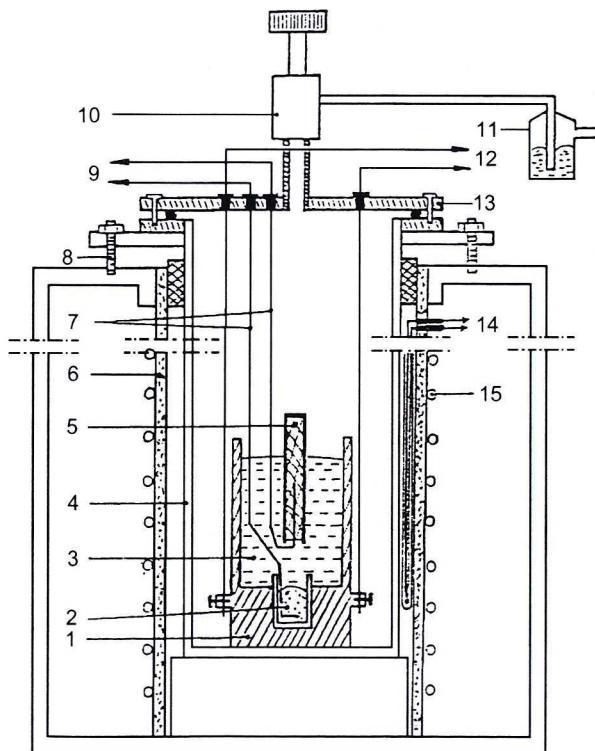
Fig. 1. Experimental arrangement used in emf studies.
