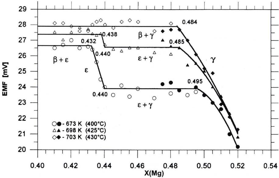
Fig. 4. Experimentally measured relation  $EMF = f[X(Mg)]$  for temperatures  $T = 673, 698$  and  $703$  K
