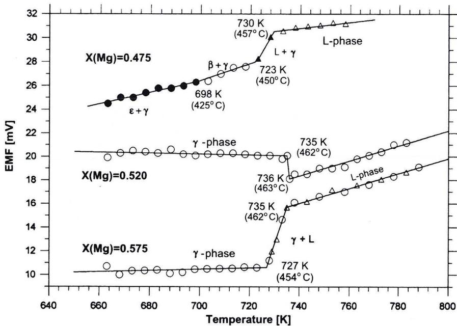
Fig. 2. Experimentally measured in [5] relation  $EMF = f[T]$  for concentrations  $X(Mg) = 0.575$  and  $0.520$ , and in this work for  $X(Mg) = 0.475$
