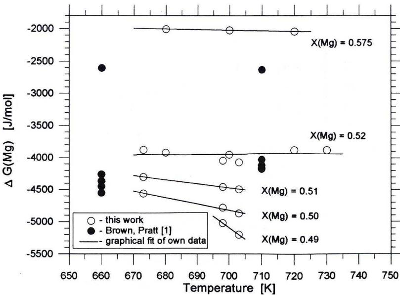
Fig. 5. The relation of partial magnesium Gibbs free energy vs. temperature. The comparison of values calculated from experimental results (with the aid of Eq. (1)) and from literature [1]
